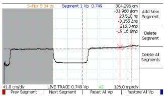
Figure 4: In this multi-cable system, the first cable has a Vp of 0.749. The other cables in this system have different Vp values. All of these values are used to produce an accurate distance-atcursor measurement.
