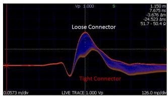
Figure 5: Intermittent fault detection with probability density plot.
