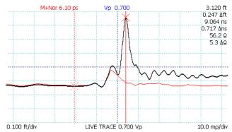
Figure 1: Comparison of normal BNC (black) vs SMA (red) connectors.
