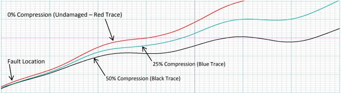
Figure 7 – Compression Damage 36 inches beyond Transformer using Adapter Type D (Zoomed in – Smoothed)
