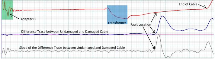
Figure 8 – Difference and Slope of the Difference Traces showing location of compression damage beyond a transformer.
