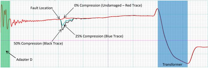
Figure 5 - Compression Damage 48 inches from Start of Cable (Before Transformer) using Adapter Type D
