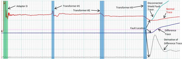
Figure 5 – Disconnected shield fault through three transformers with difference trace and derivative of difference trace for fault location
